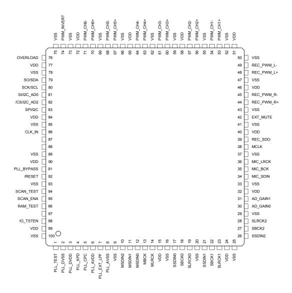
PS9702B (100pin Plastic QFP, Top View)
